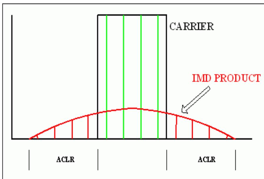
Fig.2 subcarrier model of a broadband carrier signal
