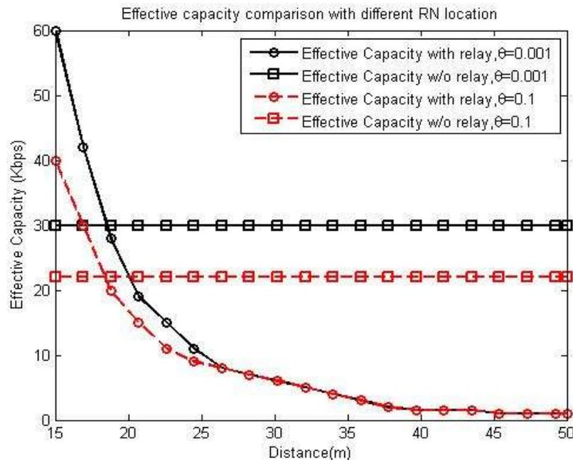
Fig.6 EC comparison with relay node and without relay node
